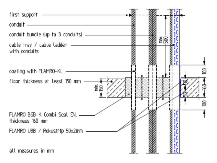
Conduits made of plastic or steel, rigid or flexible, with or without cables, outer diameter max. 25 mm
