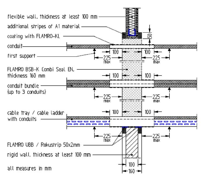
Conduits made of plastic or steel, rigid or flexible, with or without cables, outer diameter max. 25 mm
