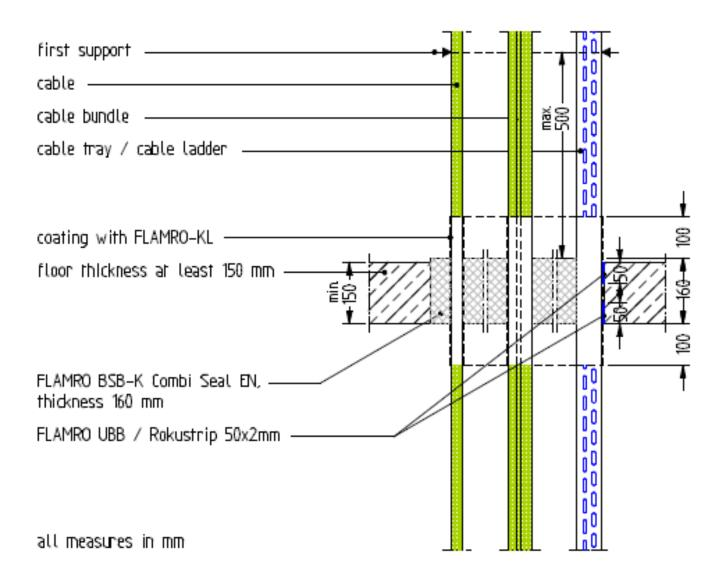
annex 6: Penetration of conduits and conduits bundles, rigid floor
