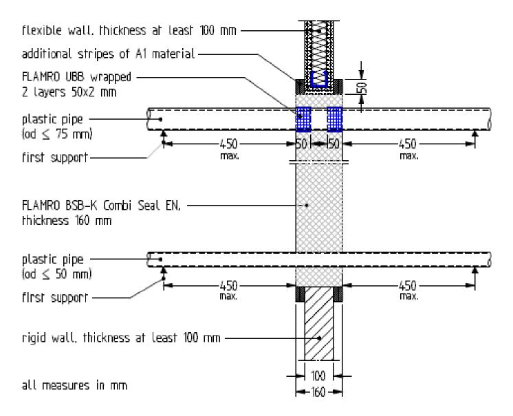
Use as part of a penetration seal. floor installation - section view
