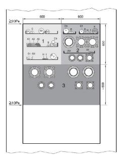
Module 1: Standard cable module Module 2: Standard mixed module
