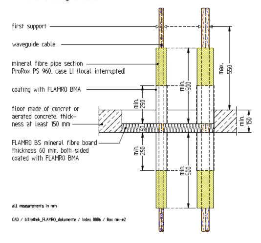
Penetration of conduits made of plastic (with and without cables)
