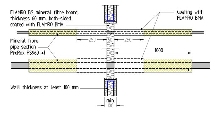
\*) mineral fibre pipe section butt-jointed to the penetration seal board (not sustained)
