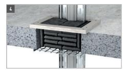
At a floor thickness of < 250 mm the floor must be doubled with non-combustible building panels to the minimum thickness of 250 mm. The steel grid at the bottom side of the opening is for installation of the fire protection pillows.
