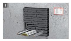
Make sure that the fire protection pillows are installed in a staggered pattern. Finally apply the label.
