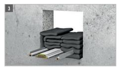
Stuff all other layers of fire protection pillows very tightly around the cables. For that purpose, the use of pillows in different sizes is recommended.
