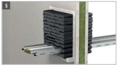
The application in lightweight partition  $\geqslant$  100 mm is possible. At a wall thickness of < 200 mm the floor must be doubled with non-combustible building panels to the minimum thickness of 200 mm.
