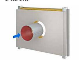
3.Close annular gap ≤ 25 mm deep on both sides with gypsum mortar (plasterboard wall); otherwise with NOVASIT BM/K2/VGM along the depth of the strutual element.
