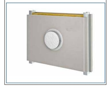
For installations in plasterboard walls with a spacing of more than 50 mm between the wall sheets on both sides of the steel support structure, the Cable Tubes have to be fixed with steel strips/wires in the region between the wall sheets.
