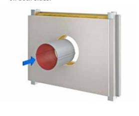
Close annular gap ≤ 25 mm deep on bothsides with gypsum mortar (plasterboard wall); otherwise with NOVASIT BM/K2/VGM along the depth of the strutual element.
