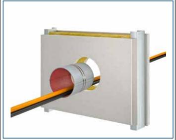
When electric wiring conduits are installed in plasterboard walls, the Cable Tubes have to be additionally fixed with a steel strip/wire on each side only for projections > 50 mm. In the region between the wall boarding, 2 steel strips/wires have to be provided.
