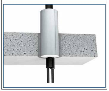
For floor installations (floor / Thickness of penetration seal  $\geq$  200 mm) two Cable Tubes CORH PYRO SF 150 connected with fabric tape can be used instead of one Cable Tubes CORH PYRO SF 300
