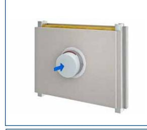
Seal the plugs completely; coat thickness ≥ 2 mm (dry coat thickness ≥ 1 mm) with FLAMMOTECT-A.
