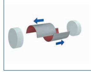
6. For connecting the Cable Tube half shells, simply press them together.
