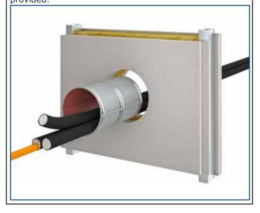
For installations in walls, the first support must be provided by the customer on both sides of the wall at a distance of  $\leq$  300 mm. The supports must be made from non-flammable construction materials.
