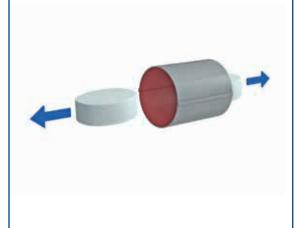
5. For separating the Cable Tube half shells, slide the shells in opposite directions.
